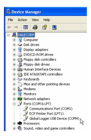
8) To confirm the installation, look in the Device Manager and find the USB Serial Port. The COM setting following that will show the virtual COM port that has been automatically assigned to the driver. As you will see in the following sections, this COM port will be automatically detected by the Global Logger software so it is not necessary to note which port is being used by the driver.
