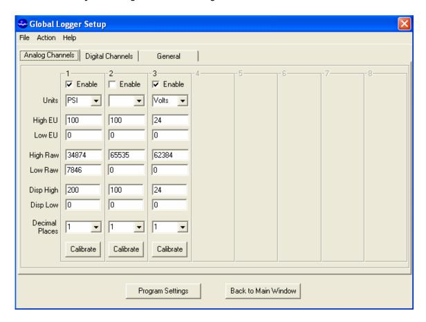
The PL200G Logger comes factory calibrated but may need re-calibration on occasion to maintain maximum accuracy. The pressure sensor is designed to measure over the range of 0-200 psi but it can be calibrated at lower pressures. The screen above shows channel one calibrated at 100 psi but set to display up to 200 psi on the main screen.
